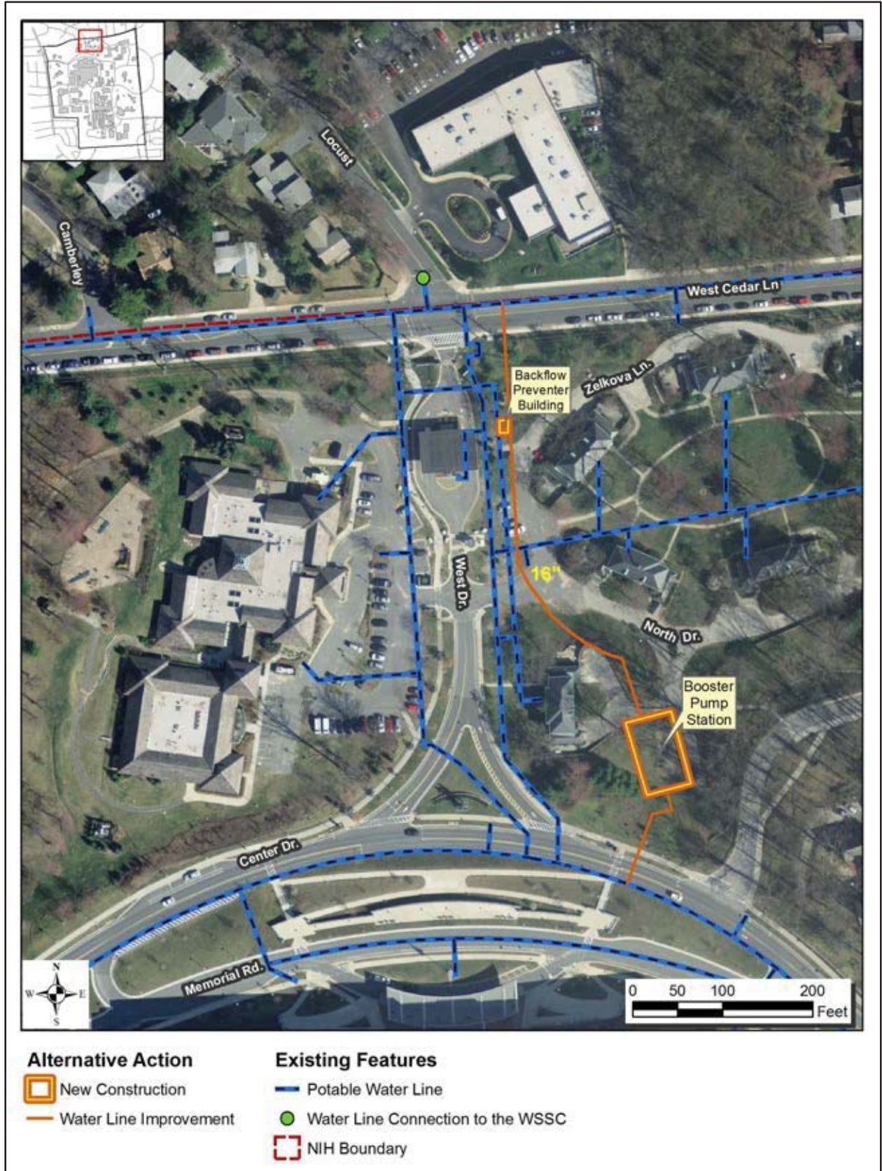
Figure 2-6. Alternative Action – Booster Pump Station and Backflow Preventer
