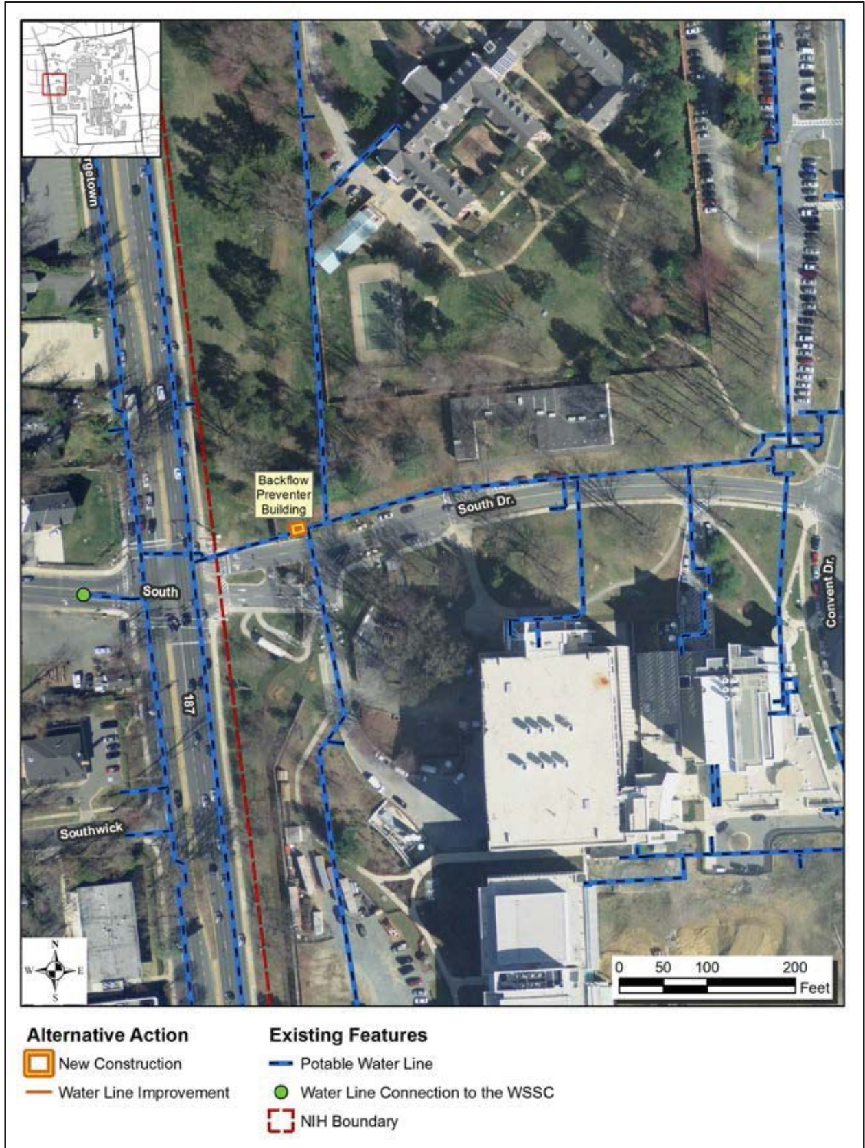
Figure 2-8. Alternative Action - Backflow Preventer Near South Drive
