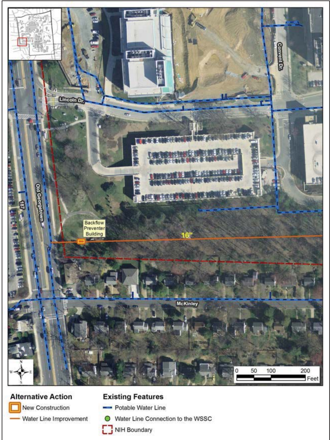
Figure 2-9. Alternative Action – Backflow Preventer Near Lincoln Drive
