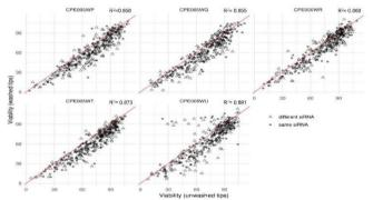
Two sets of assay plates were screened against the Ambion Silencer Select Human Kinase siRNA library to validate the effectiveness of the tip washer. The first set was processed with new sterile tips while the second set was processed using tips cleaned with the TipNovus Mini. Validation assay protocol was then
