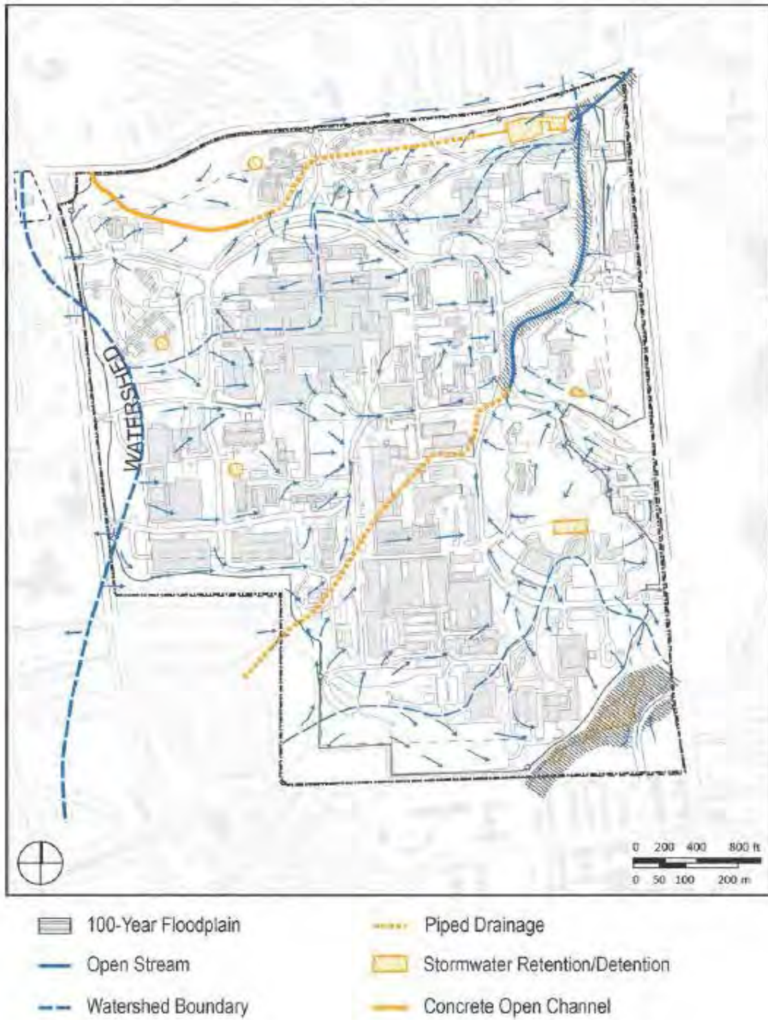
Figure 3.4-2. Stormwater System, Drainage Sheds, and Floodplains on the Campus
