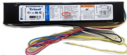
A typical Non-PCB containing fluorescent light ballast. The ballast has a "No PCBs" marking on the top of the ballast and the text "electronic ballast". Only magnetic fluorescent light ballasts contained PCBs.
